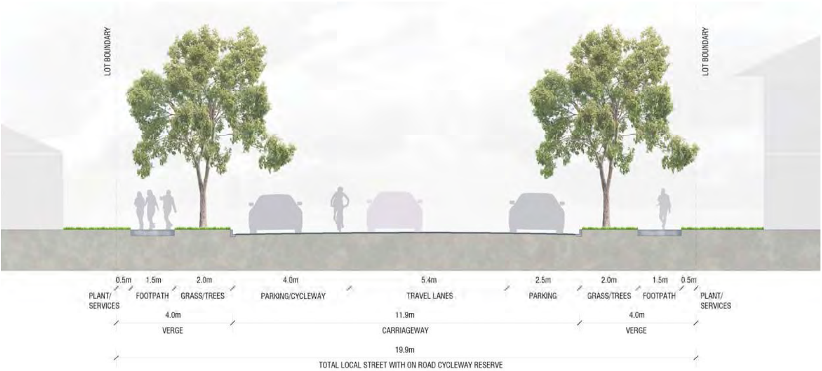
LOCAL STREET WITH ON ROAD CYCLEWAY
